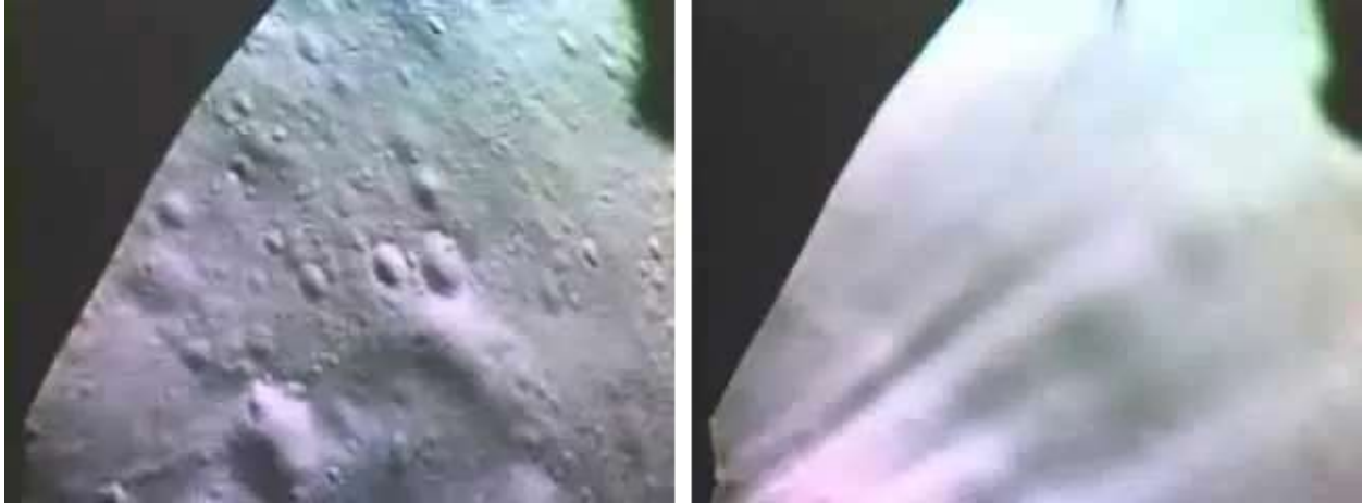
Figure 1: Frames from video footage of Apollo 15 landing showing difference between clear view of ground (left) and view obscured by PSI effects (right)
