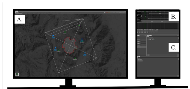
Fig 1. Ground control station setup, consisting of two displays, Tactical Situation Display (TSD, A.) on the left side and the Timeline (B.) HAT Assistant (C.) on the right side.
