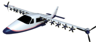
Mod IV - Design for low-speed takeoff and landing characteristics with an integrated Distributed Electric Propulsion (DEP) system.
