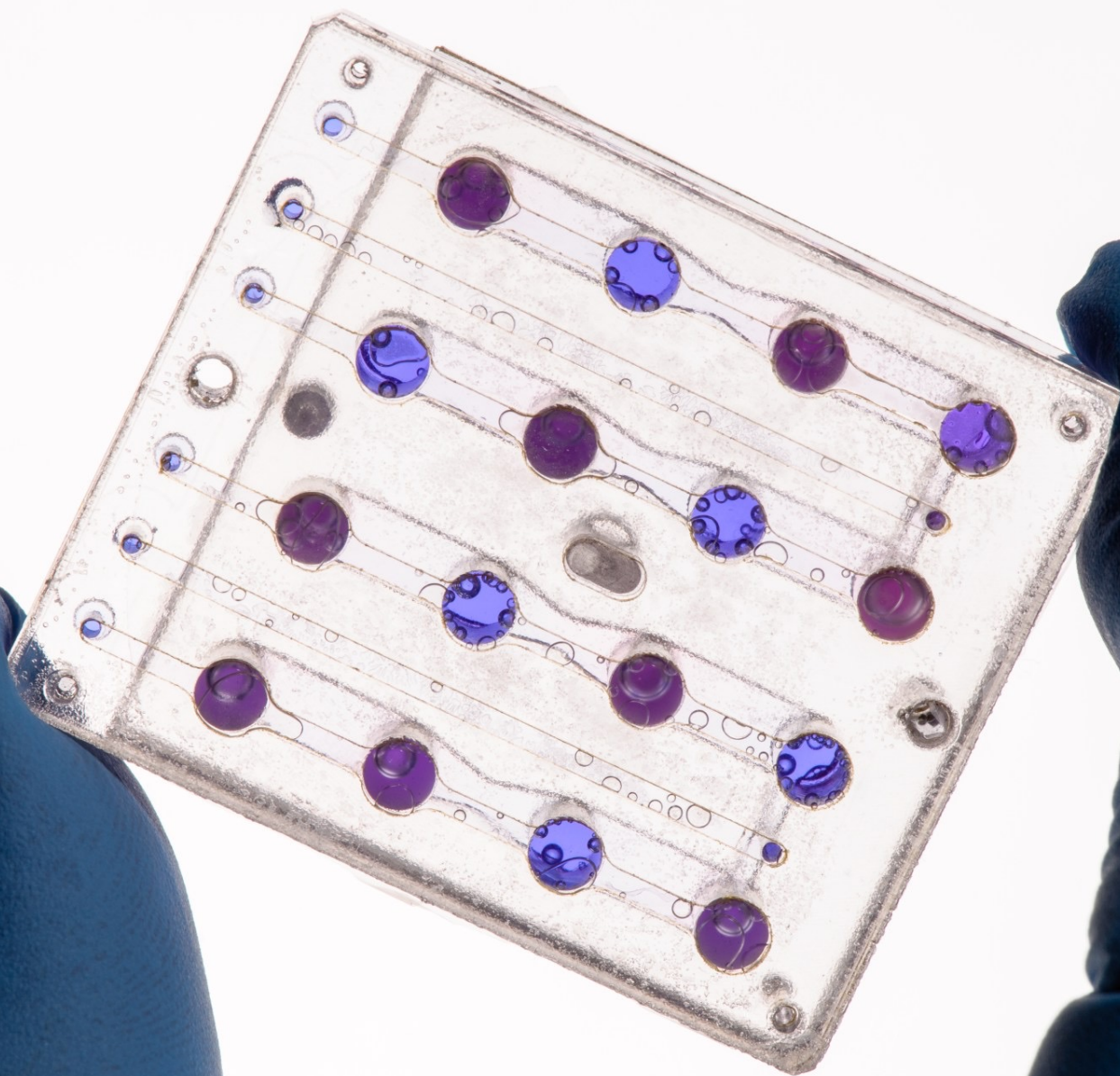
Fluidic card with yeast, BioSentinel mission. image credit: NASA
