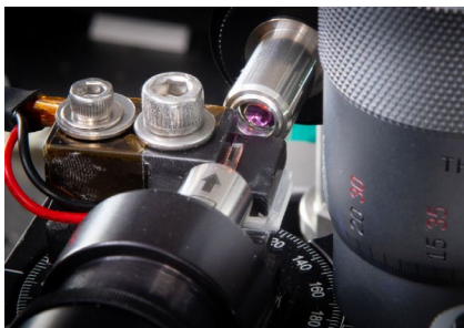
Waveguide SPDC source
