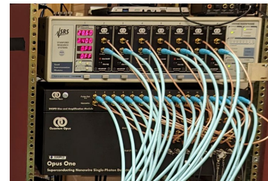
Rack-mounted SNSPD cryogenic system
