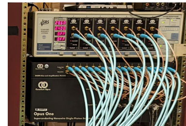
Rack-mounted SNSPD cryogenic system
