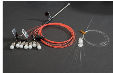
Fully packaged photonic lantern
