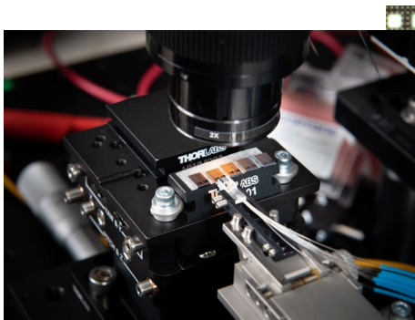
Integrated photonic chips on probe station
