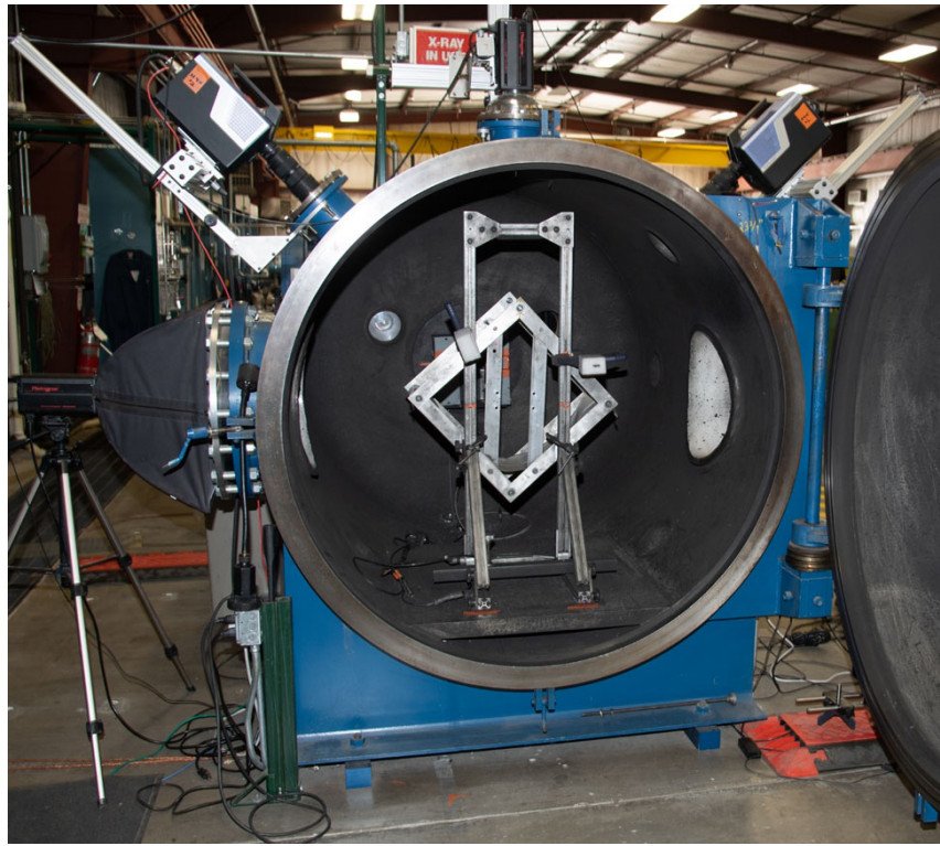
Fig. 1. High-speed imaging setup using frame-synchronized, ultrahigh-speed Shimadzu™ HyperVision HPV-X cameras located outside the target chamber.
