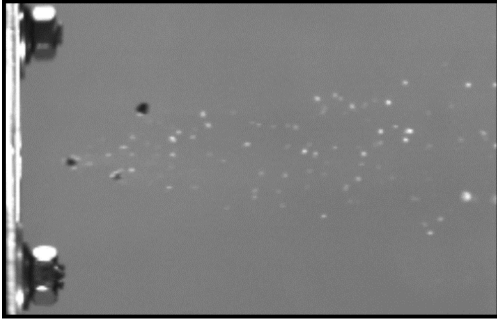
Fig. 2. Image of first 6 x 1.2 mm CFRP disk breakup machined from CFRP sheet with a length-to-diameter ratio of 1/5.
