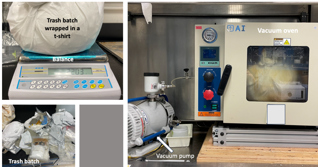
Figure 4. Trash model example used for moisture analysis using heat and vacuum (photo credit NASA ARC)
