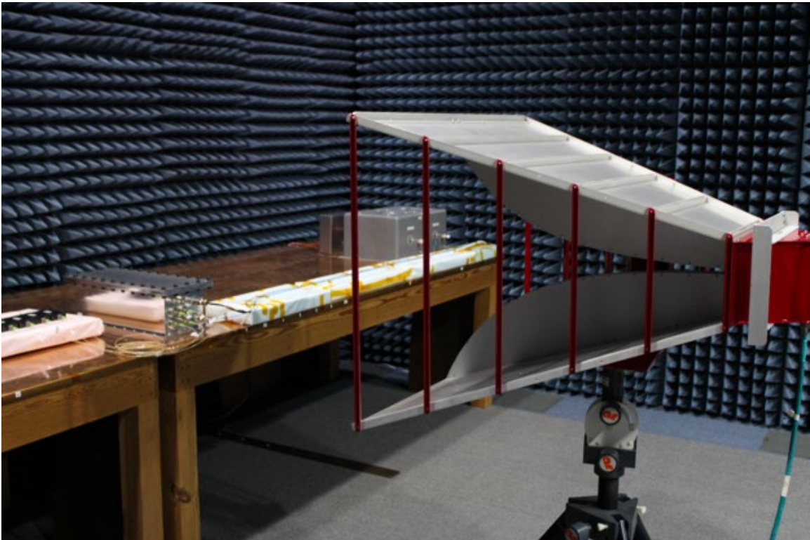
Fig. 19 FOSS undergoing RE 102 testing within a range of 200 MHz-1 GHz.
