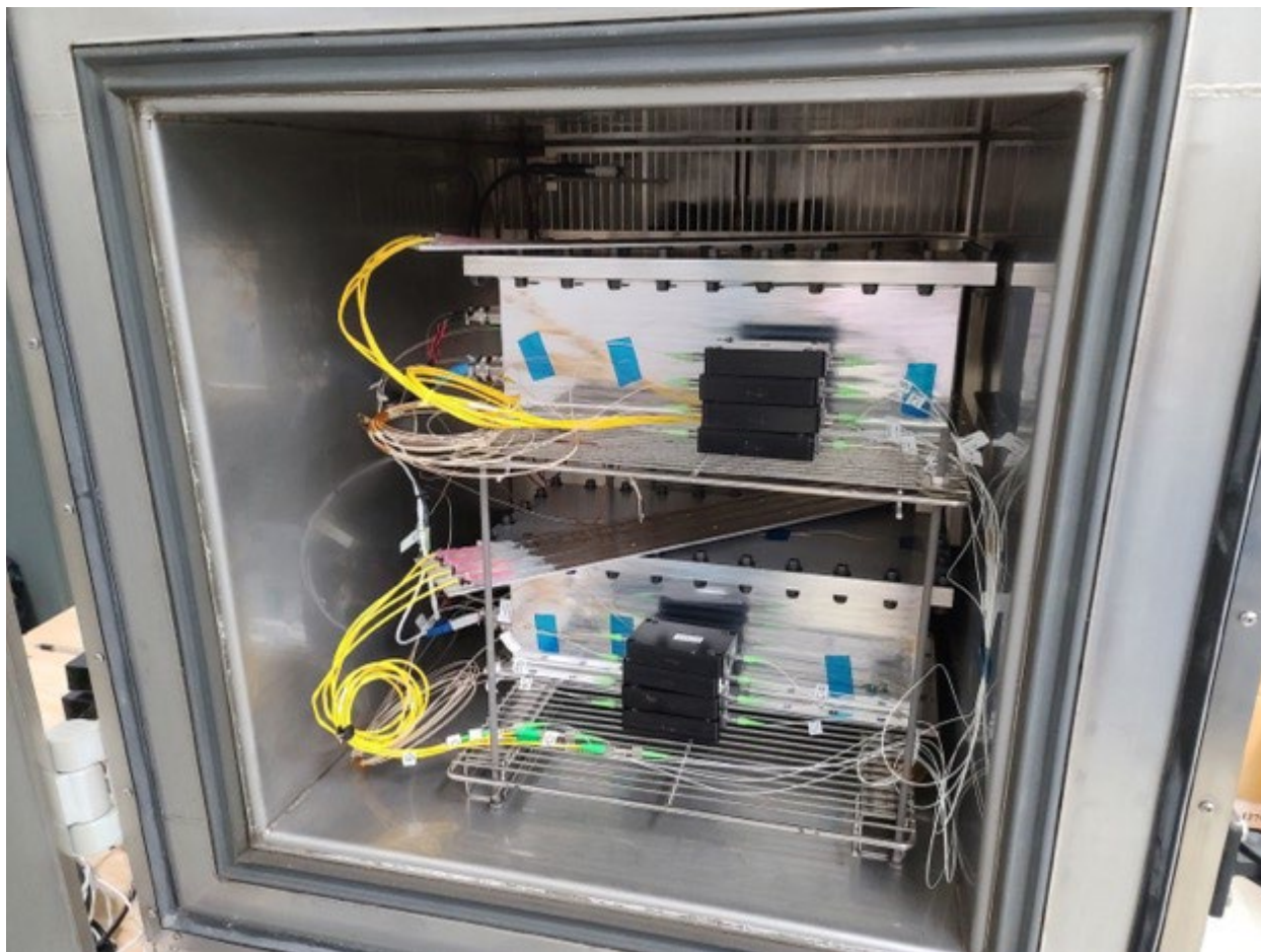
Fig. 15 FOSS units inside a thermal chamber prior to undergoing thermal cycling at NASA KSC.
