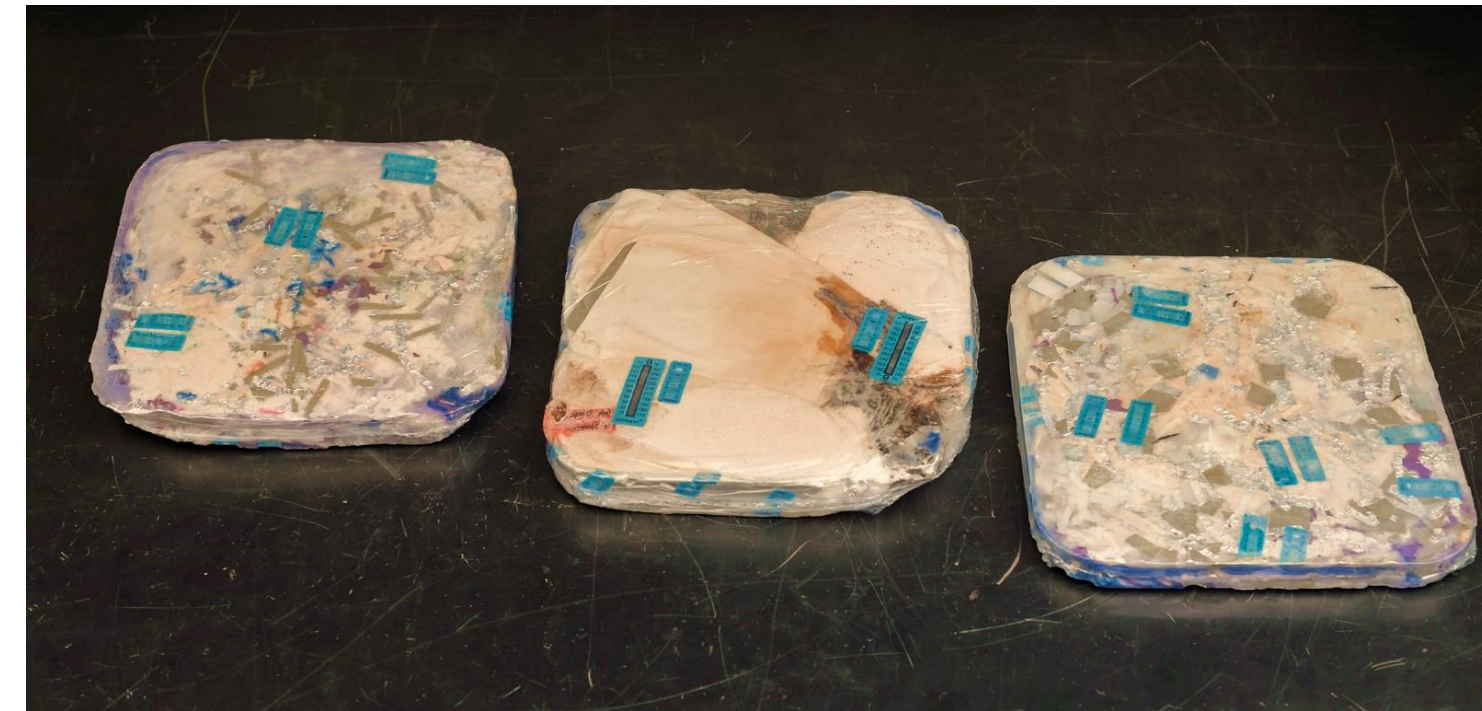
Figure 8. Trash tiles produced in the Gen 2 TCPS
