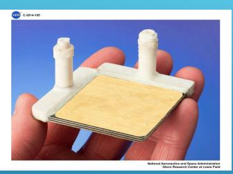
SOFC/SOEC – Lunar/planetary power & ISRU, terrestrial carbon capture & hydrogen economy.
