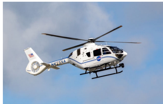
Fig. 3(b) The helicopter data collection platform: Airbus H135 with WESCAM MX-10. (NASA photograph number KSC-20201027-PH-KLS01_0040.)
