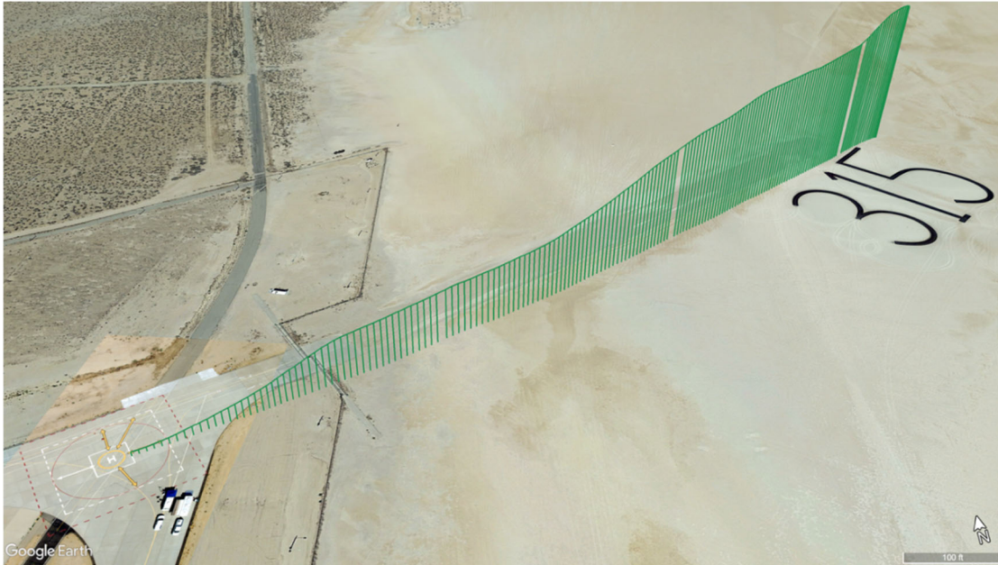
Fig. 4 Example segment of the sUAS approach trajectory landing at the NASA Armstrong Flight Research Center 01H helipad starting at an altitude of 250 ft (76 m) and 1500 ft (460 m) downrange.
