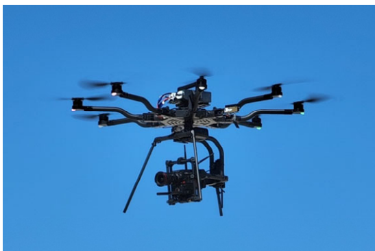
Fig. 3(a) The sUAS data collection platform: Freely Alta 8 sUAS with a RED DSMC2 camera mounted on a Movi Pro gimbal. (Photograph courtesy Nelson Brown, AFRC.)
