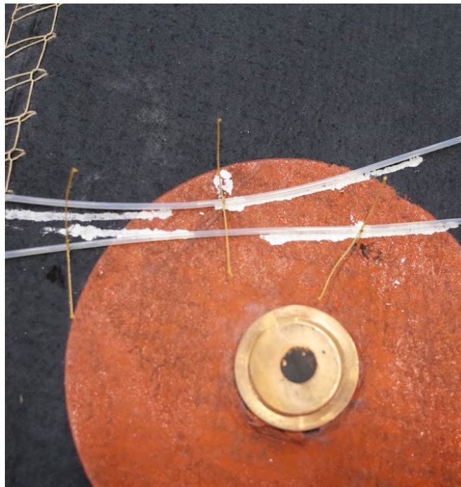
Fig. 3 Loose PTFE sleeve containing temperature sensing FBGs, being held in place by loose threading, which is located between the FTPS layers.
