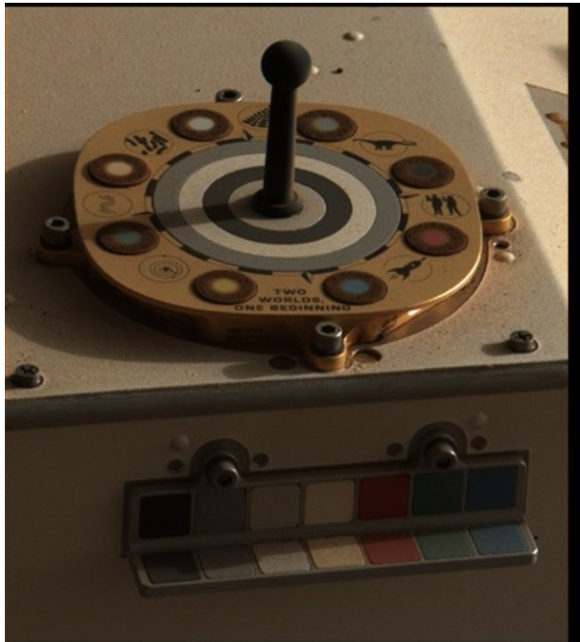
Figure S11: Subframed image of the Mastcam-Z radiometric calibration targets (55) acquired by Mastcam-Z through the left-eye broadband (L0) filter at 48-mm focal length on sol 236 in late afternoon (sequence zcam03014). This low-sun frame shows the thick dust rings attracted to the eight strong magnets as well as the relatively clean spots at the center of each patch where the magnetic force repels magnetizable dust. The top surface of the primary target (top) is 10 cm across and the top of the gnomon is 3.75 cm above that surface. The secondary target (bottom) is 8 cm long. The primary target is embellished with a variety of education and public outreach elements (70).
