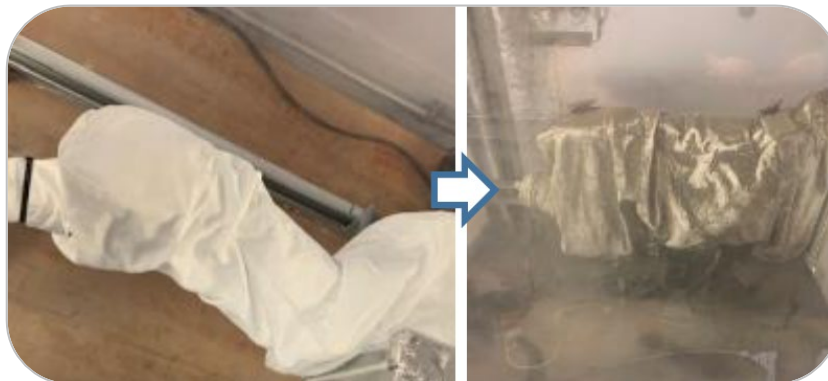
VIPER Wheel Assy Dust Exposure Test
