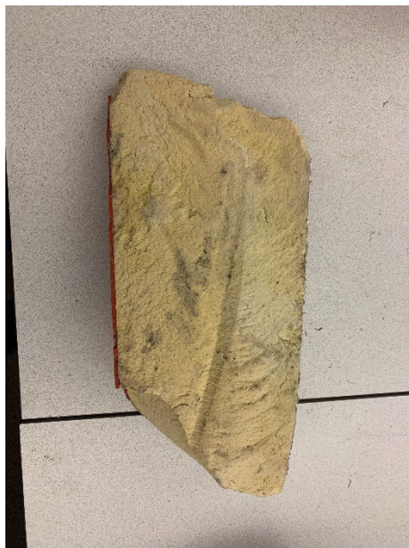
Fig. 3 Booster Throat Plug Fragment Recovered after Artemis I
