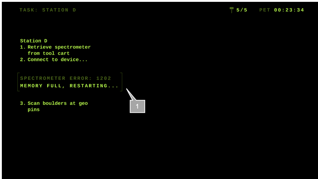
Figure 6.47: Annotated Joint AR user interface solution that addresses the momentary demand: "I want to know what a fault indication means"
