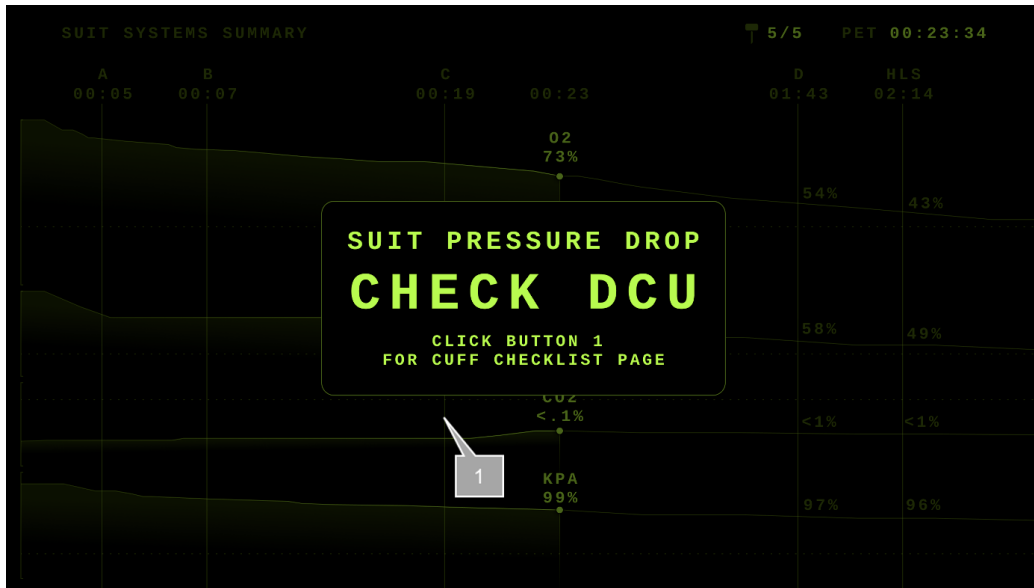
Figure 6.32: Annotated Joint AR user interface solution that addresses the momentary demand: "I want to see a visual cue of an alert"
