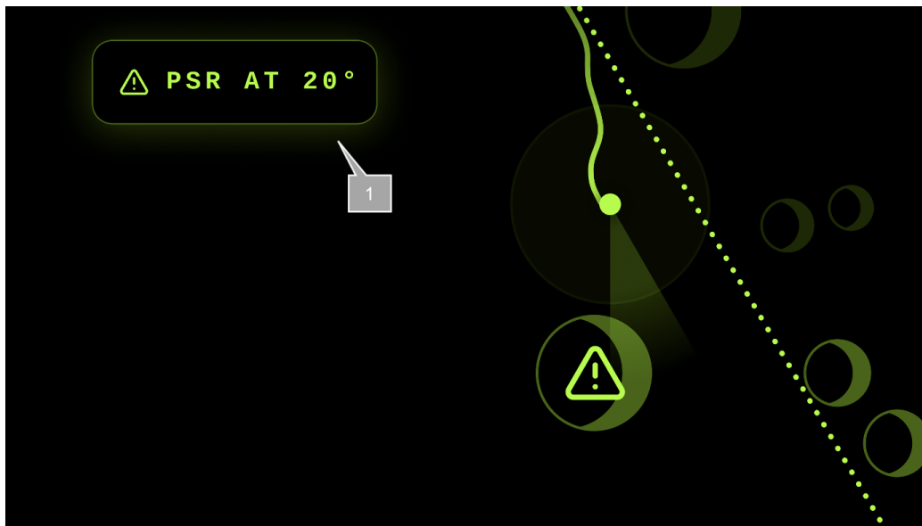
Figure 6.34: Annotated Joint AR user interface solution that addresses the momentary demand: "I want to receive caution or warning notifications related to sensitive or hazardous environments or equipment that could be inadvertently disturbed while completing the current task"
