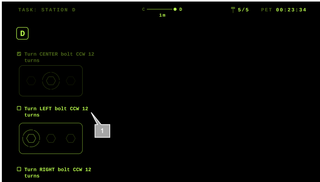
Figure 6.43: Annotated Joint AR user interface solution that addresses the momentary demand: "I want to maintain situation awareness of current and completed procedure steps"
