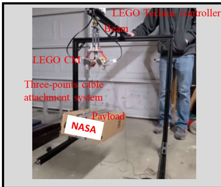
Figure 6. Validation of single cable leveling control system.
