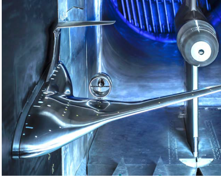
Figure 5 – KNOPTER/CDISC designed Hybrid Wing Body in the NTF. [Photo: NASA from Ref. 73].
