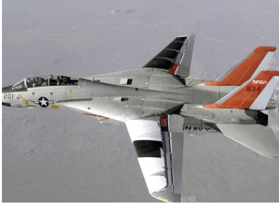
a) Test aircraft with NLF gloves. [Photo: NASA]
