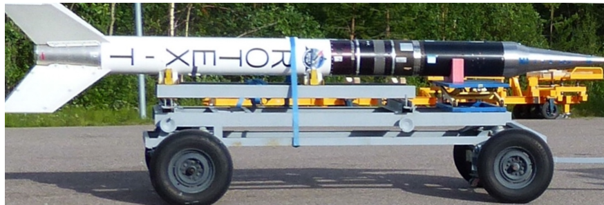
Fig. 1 Photograph of the ROTEX-T payload mounted to the second stage [Source: DLR].
