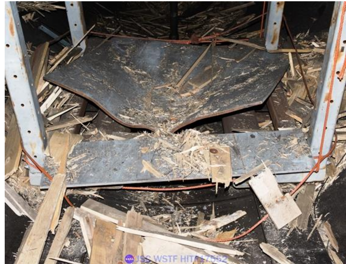
HVIT17552: 5.0mm Al @ 6.82 km/s, 0deg (note: buckling of 5/8" thick steel plate under the test article)
