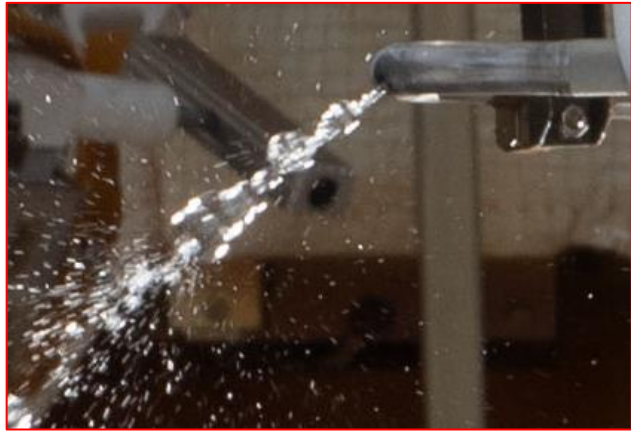
Iss070e006528: MLM Radiator Line Leak Location
