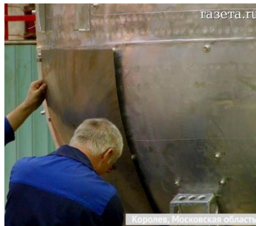
Bumper shield and Standoffs being added to outside of Soyuz Orbital Module and Progress Cargo Module.
