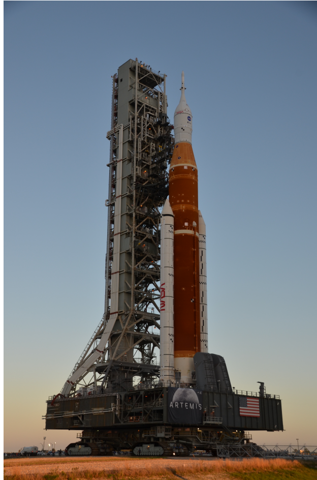
Fig. 2 First SLS Block 1 vehicle rollout to Pad 39B on March 17th, 2022, showing the SLS launch vehicle, the Mobile Launcher (ML) and the Crawler-Transporter (CT) [Source: NASA, Pinier].
