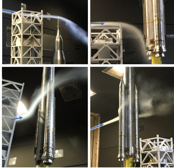
Fig. 13 Smoke flow visualization of a scaled liftoff SLS Block 1B crew vehicle model and the mobile launcher. Flow direction is indicated by the blue arrows [Source: NASA].
