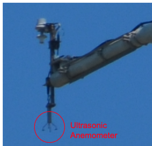
Fig. 4 Photograph of an ultrasonic anemometer installed on one of the lightning towers [Source: NASA, Pinier].
