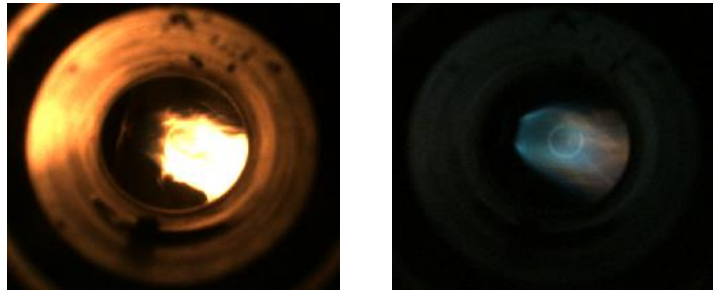
Fig. 5. Images of typical flames from Jet-A (left) and sustainable aviation fuels (right) in the PAL combustion chamber. Flow is left to right. The circular shaped object that can be seen through the blue flame is the spark plug mounted on the opposite side of the chamber from the camera.
