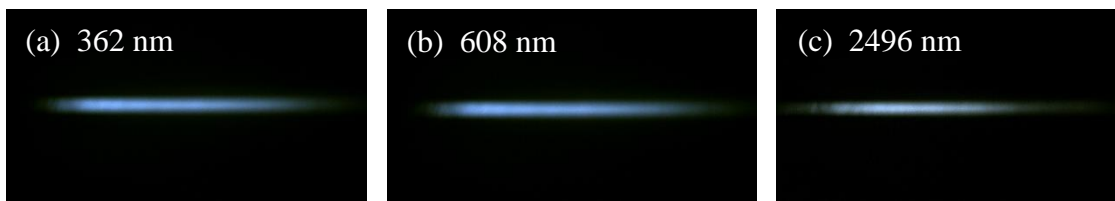
Fig. 9. Camera images of the illuminated plume observed from 90° for various sizes of ice particles.
