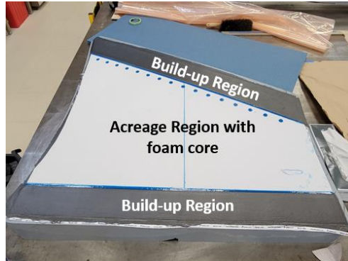
Fig. 8. Wing skin cross sectional and internal view of build.
