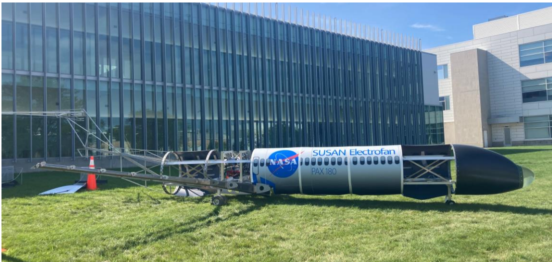
Fig. 6. Completed fabrication of 25% manufacturing demonstration vehicle.
