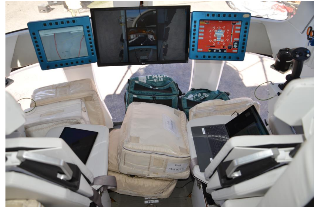
Cockpit layout with windows exposed and control screens active (Note: stowage bags temporarily stowed in pilot/co-pilot driving area for EVA)
