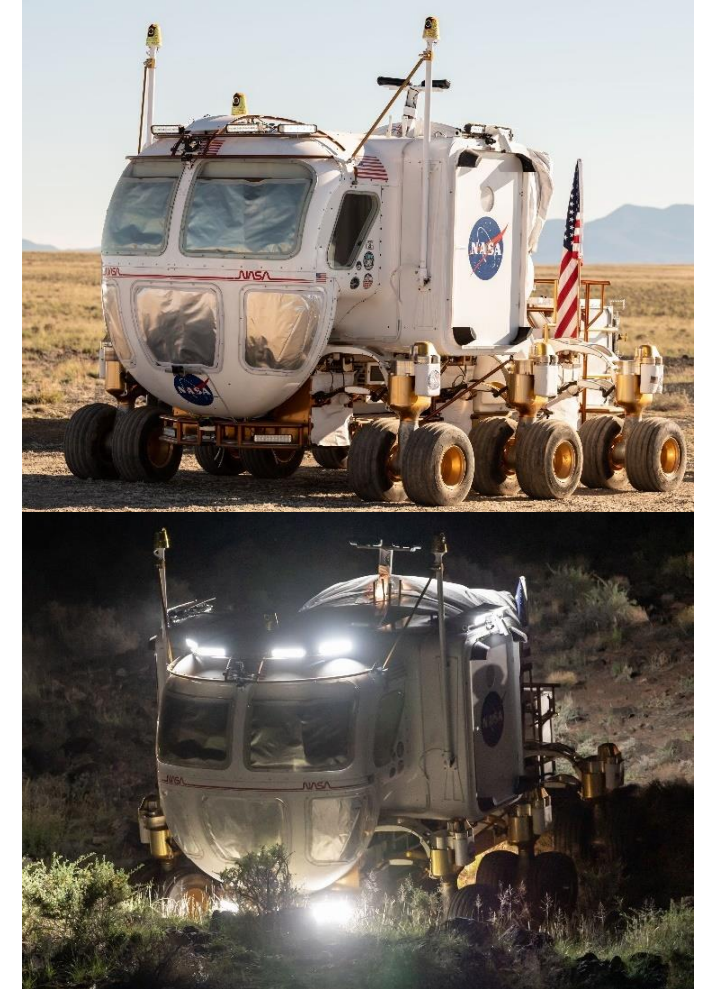
GEN 1B PR testbed in “drive-by-cameras” driving mode with windows covered during a day test (top image) and a night test (bottom image)
