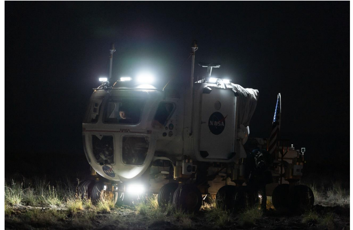
Crew driving analog PR at night with windows exposed using exterior lights for driving and IVA Observations
