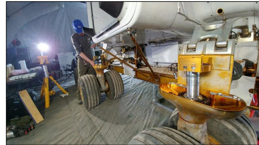
Rover team member servicing rover steering unit in tent
