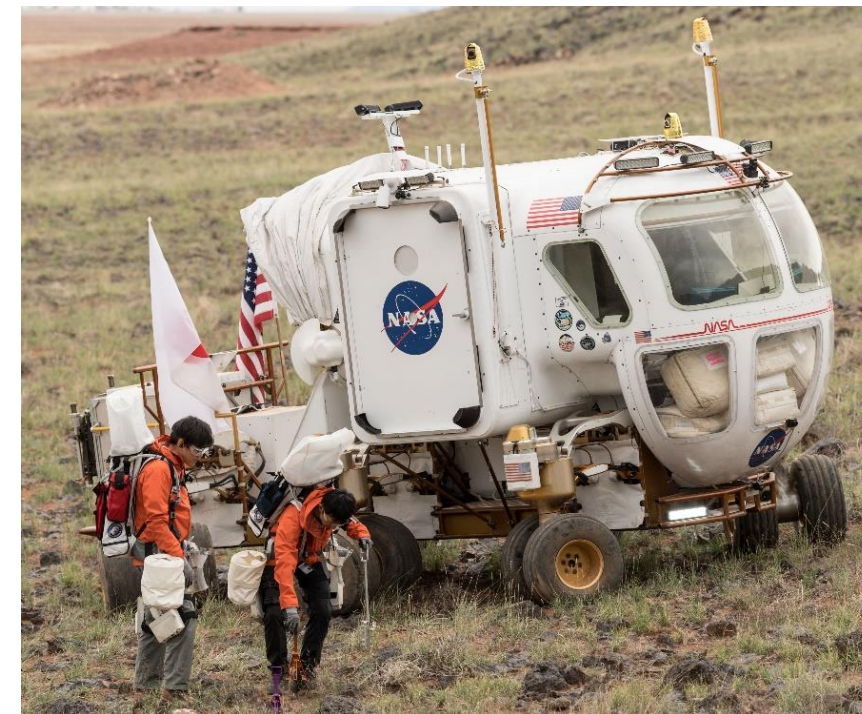
PR analog with soft cargo storage bags visible in cabin (when simulating EVA, crew must move cargo away from hatch into driving compartment to egress)
