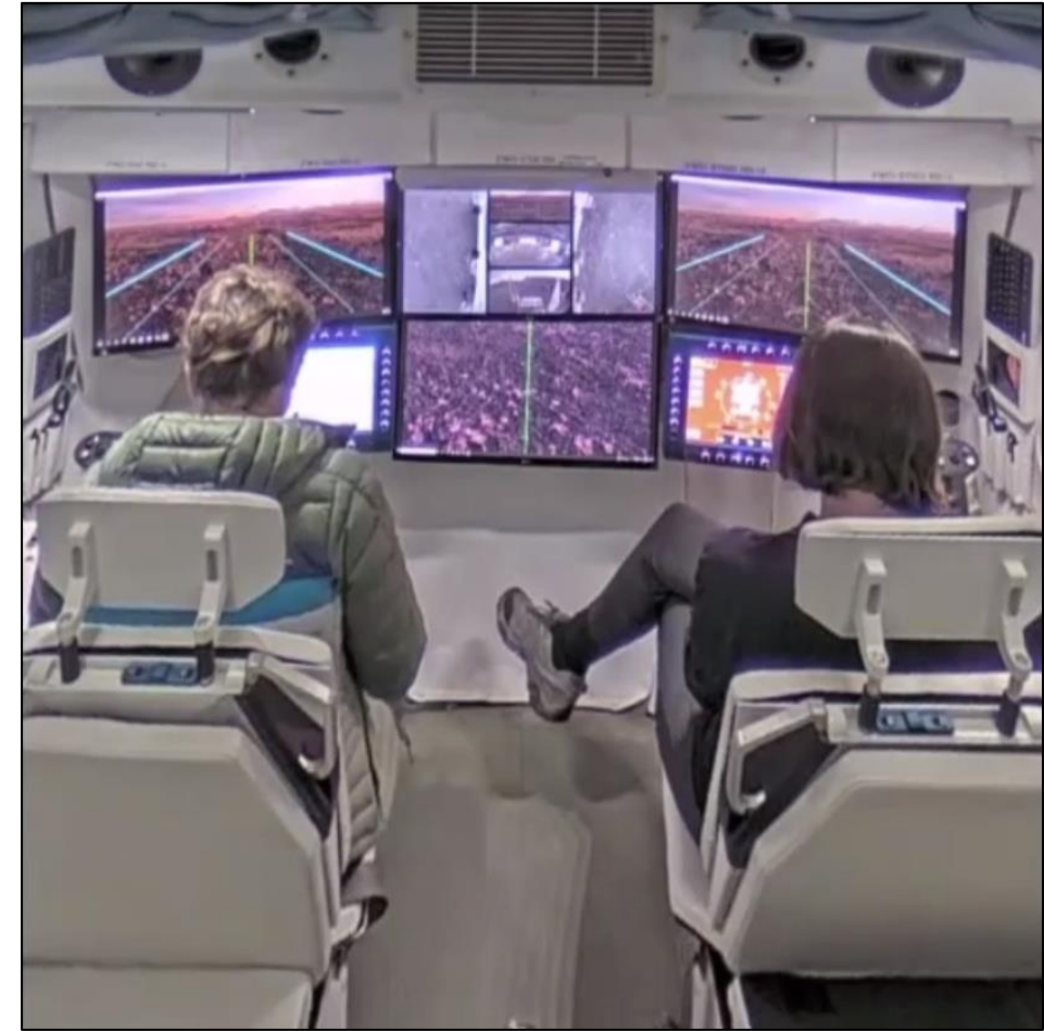
Crew driving in “drive-by-camera” mode, using bank of monitors as their guide
