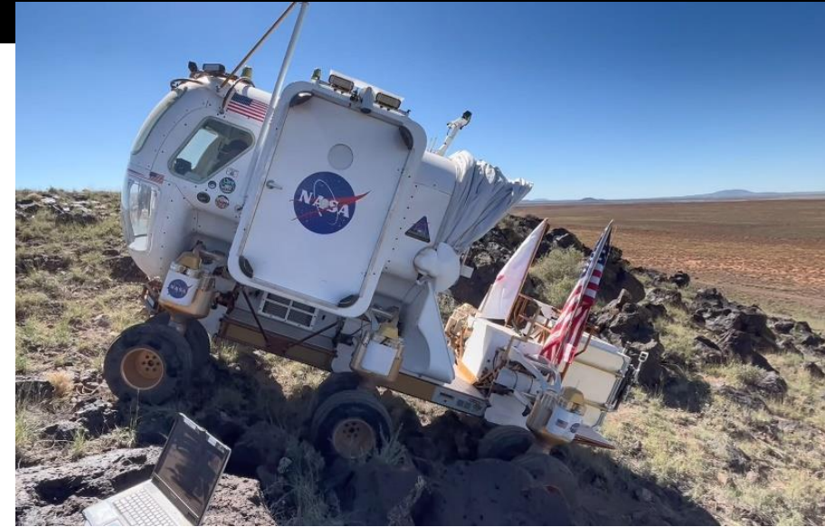
Rover analog testbed climbing ~20-degree, rocky hill
