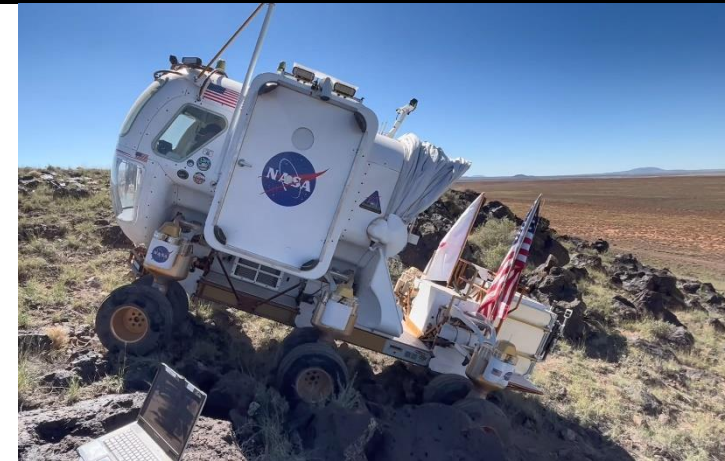
Rover analog testbed climbing ~20-degree hill
