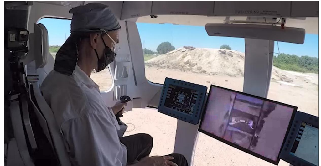
“Drive-by-windows” mode configuration – large open windows with a single situational awareness (SA) screen flanked by pilot and copilot instrument panels
