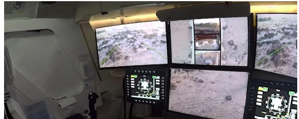
“Drive-by-camera” mode configuration - windows covered and three internal displays added, which displayed exterior driving camera views (SA view displayed on center top screen)
