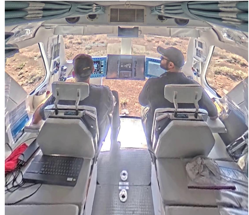
Engineering crew driving in the tested Drive-by-Windows configuration
