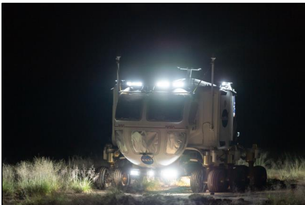
Driving rover in drive-by-camera mode at night w/ windows blacked out
