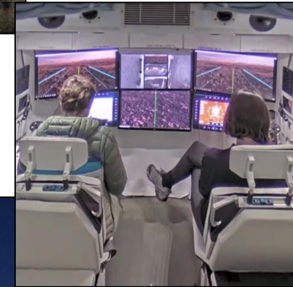
Crew driving in "drive-by-camera" mode, using a bank of removable driving monitors as their guide
