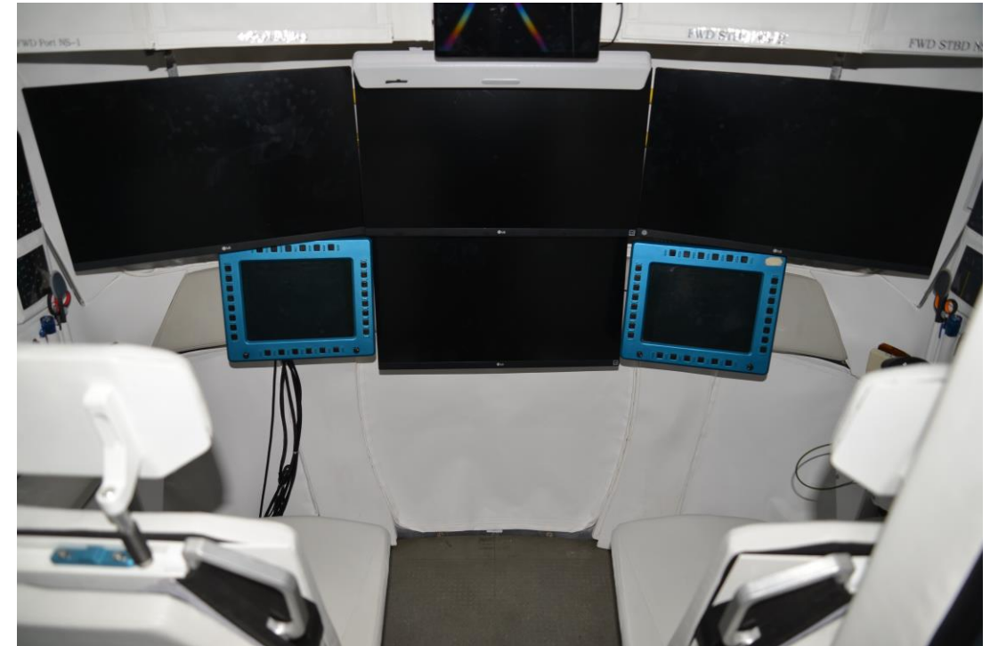
Cockpit layout with windows covered and driving screens installed
