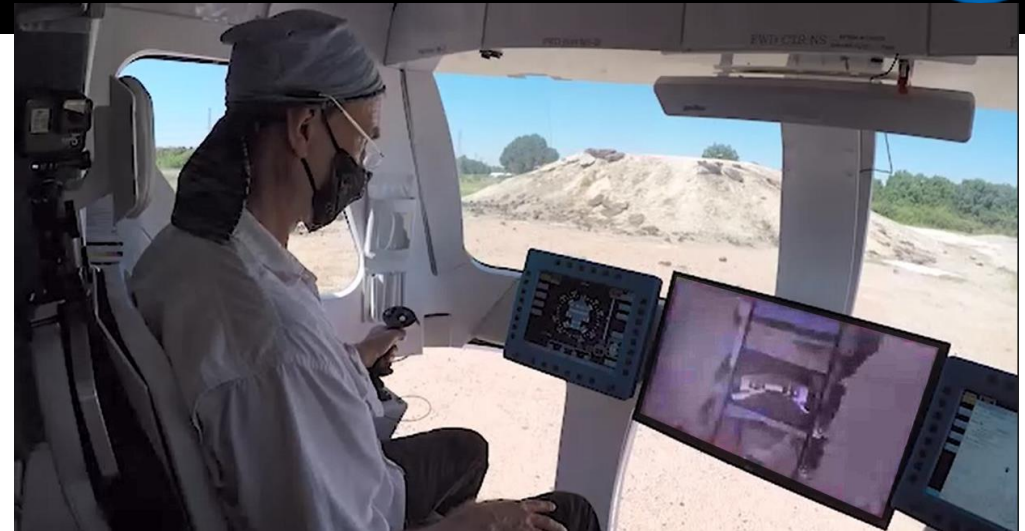
“Drive-by-windows” mode test setup – large open windows with a single situational awareness (SA) screen flanked by pilot and copilot instrument panels
