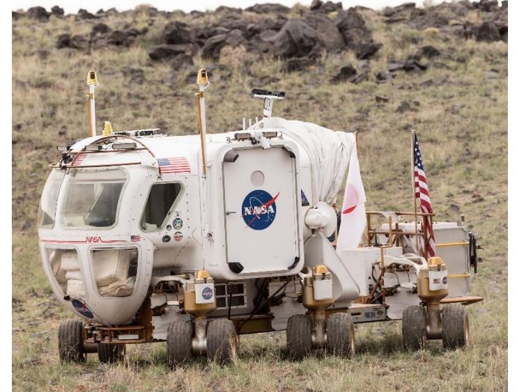
PR testbed demonstrating crabbing at ~45 degrees (rover is moving towards the camera while the nose is pointed 45 degrees to the left of the viewer)
