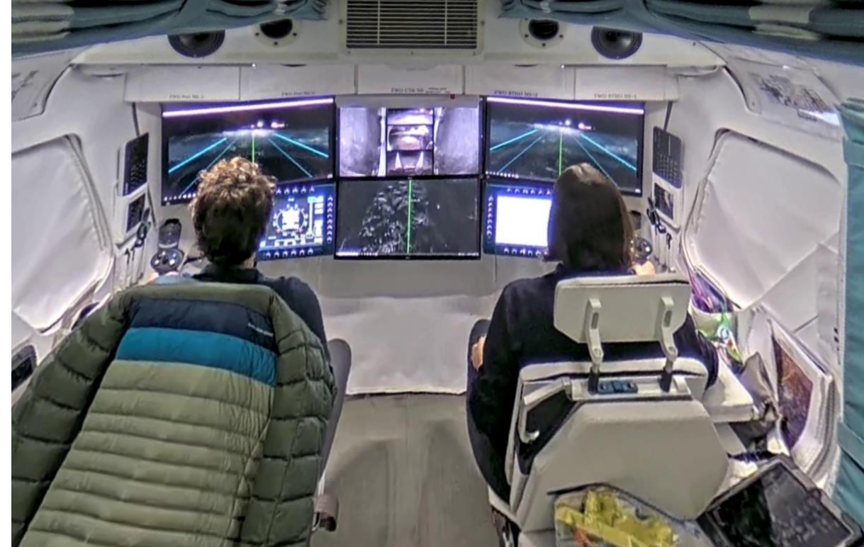
Crew driving in the tested Drive-by-Camera configuration
