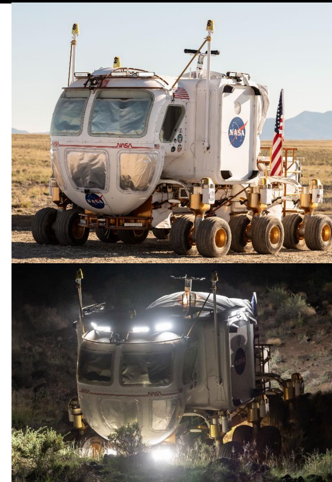
NASA's GEN 1B pressurized rover (PR) testbed was updated to include a "drive-by-cameras" driving mode, shown here with windows blocked in day (top) and night (bottom) tests
