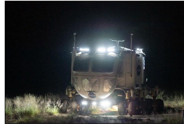
Driving rover by cameras at night with all windows covered/blacked out and flood lights on
