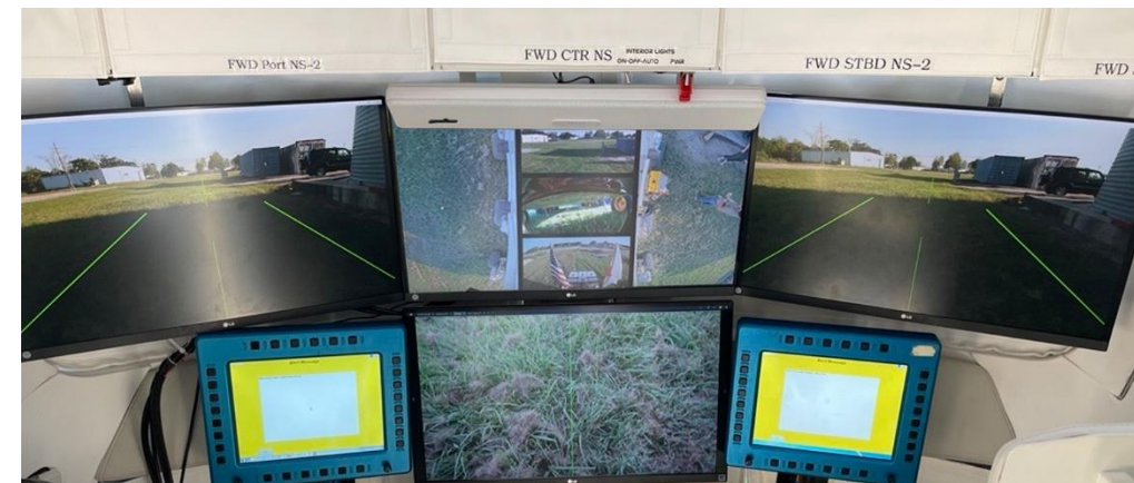
Interior view with displays configured in default drive-by-camera mode
