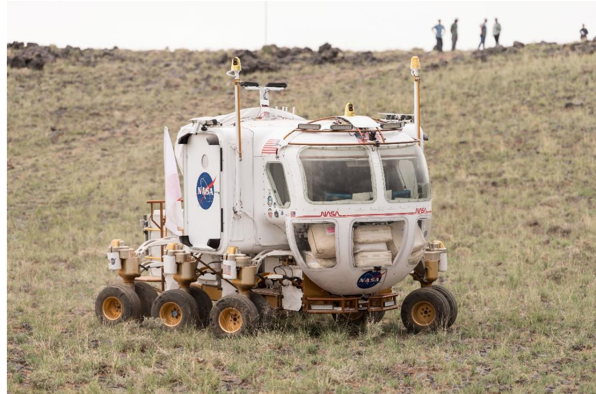
Analog PR driving at a 45-degree crab angle during teleoperation
