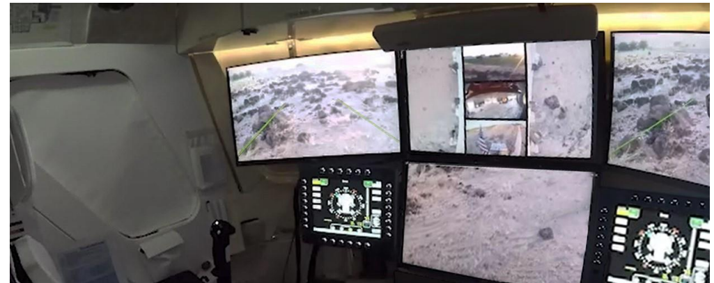
“Drive-by-camera” mode test setup - windows covered and three internal displays added, which displayed exterior driving camera views (SA view displayed on center top screen)
