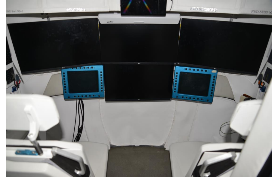
Interior view with windows covered and driving screens installed
