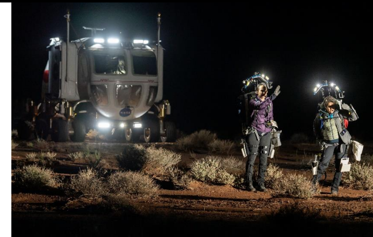
Simulated low-angle sunlight/long shadows at lunar poles by testing at night with portable, high-intensity light
