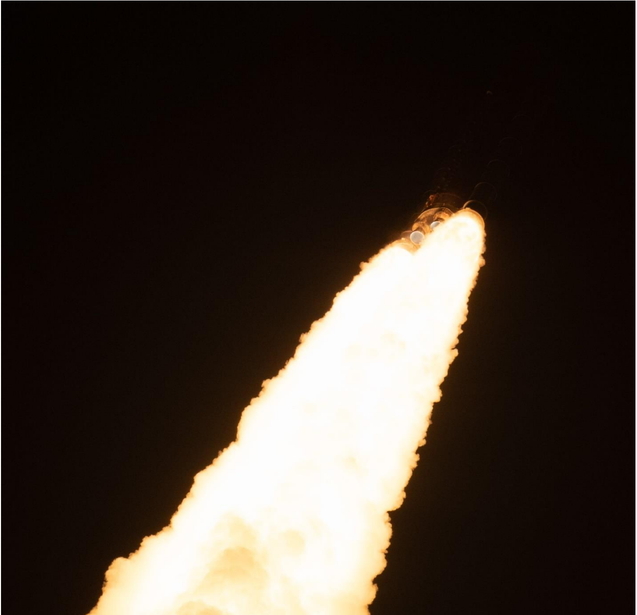
Fig. 4 The Artemis I SLS's twin solid rocket boosters and four RS-25 engines propel the rocket and spacecraft for the first time on Nov. 16, 2022.
