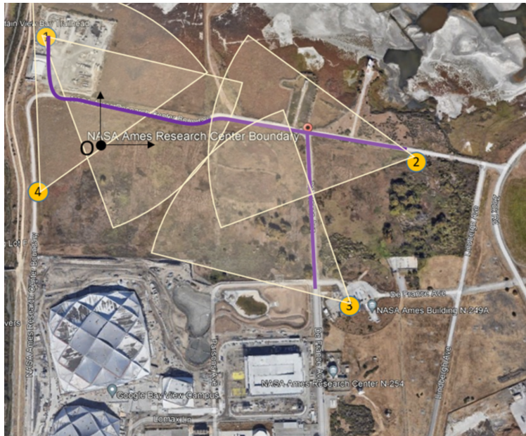
Fig. 20 Ames Research Center Flight Test - Build 1: Google Earth - approximate sensor station locations (yellow), origin (black dot), & UAS path (purple line) [31, 34]
