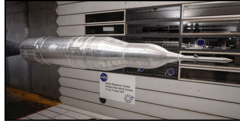
(d) Block 1B crew 4%-scale RBM tested during the ARC UPWT AUAT.
