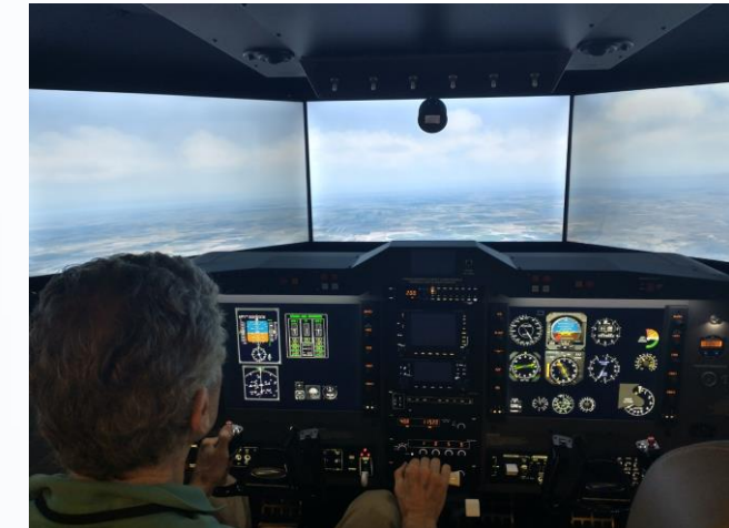
Piloted flight simulator evaluation of powertrain fault modeling and recovery, and certification-type testing
