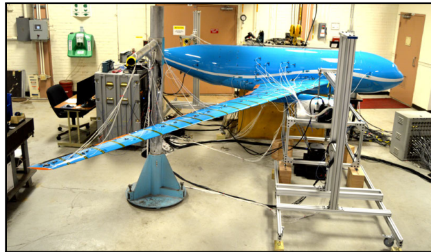
Fig. 10 WT test article instrumented with external accelerometers during the backstop GVT [Source: NASA].
