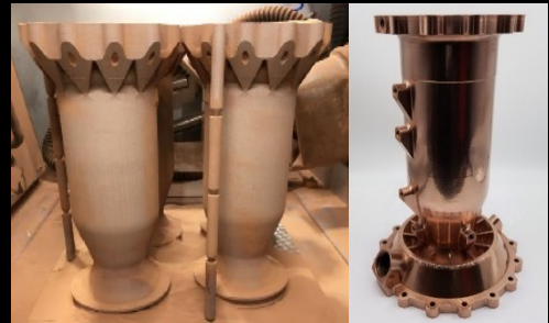
Laser Powder Bed Fusion (L-PBF) GRCop42. Courtesy Dr. Dave Ellis (NASA GRC).
