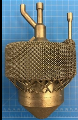
L-PBF AM IN718 TVS Augmented Injector. Courtesy Travis Belcher (NASA MSFC).
