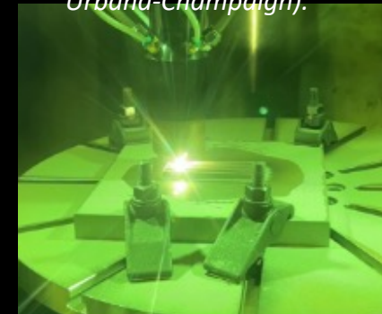
LP-DED AM C103 development. Courtesy Univ. of Texas, El Paso (UTEP).
