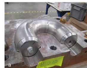
J-2X Rocket Engine Gas Generator Duct: a) Traditional tooling, b) L-PBF part
