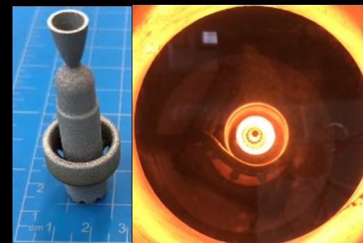
L-PBF AM W chamber test at 1900 °C. Courtesy Dr. Jamelle Williams (NASA MSFC).
