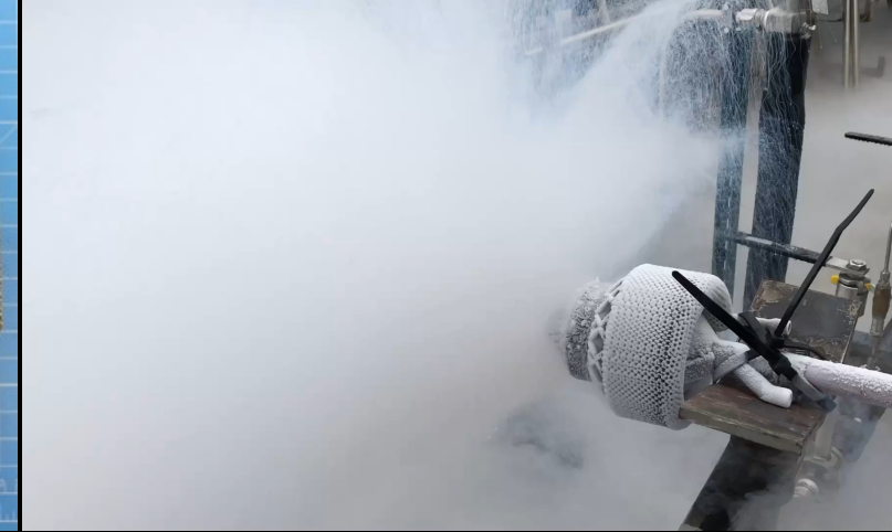
L-PBF AM IN718 TVS Augmented Injector. Courtesy Travis Belcher (NASA MSFC).
