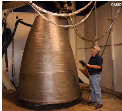
2.41 m dia and 2.82 m height Near Net Shape Forging Replacement
