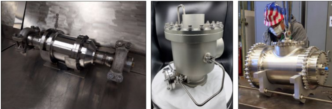
Fig. 5 Low-Leakage Test Valves: LLIV (Left), LLRV (Center), LPV (Right)
