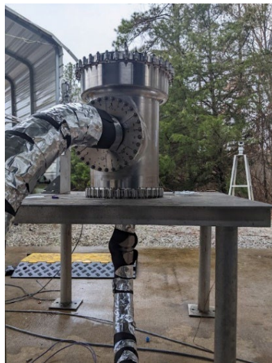
Fig. 41: LPV Prior to LH 2 Test
