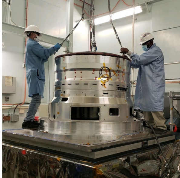
Fig. 5 Inflation System Vibe Test Configuration
