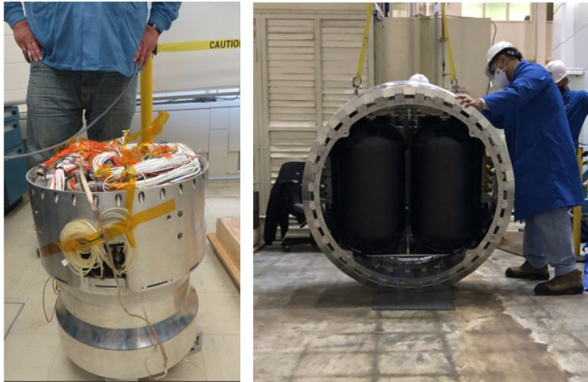
Fig. 2 IRVE-3 Centerbody (Left) vs LOFTID Centerbody (Right)
