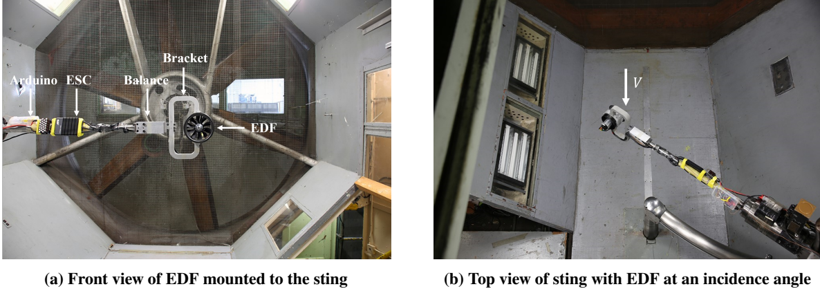
Fig. 4 Experimental setup in NASA Langley 12-Foot Low-Speed Tunnel.
