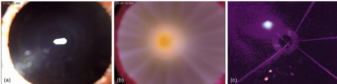
Fig. 15 Images from the uplook camera video during (a) separation, (b) atmospheric entry, and (c) parachute deployment.
