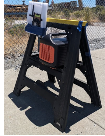
(b) Ground node with RF antenna
