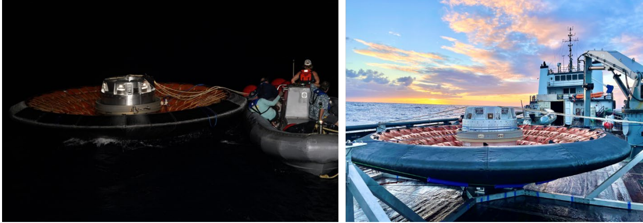
Figure 11: RV Floating in the Ocean and Aboard the Recovery Ship
