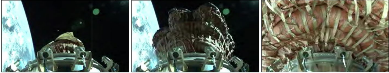
Figure 8: Packing Restraint Release to Deploy the Aeroshell
