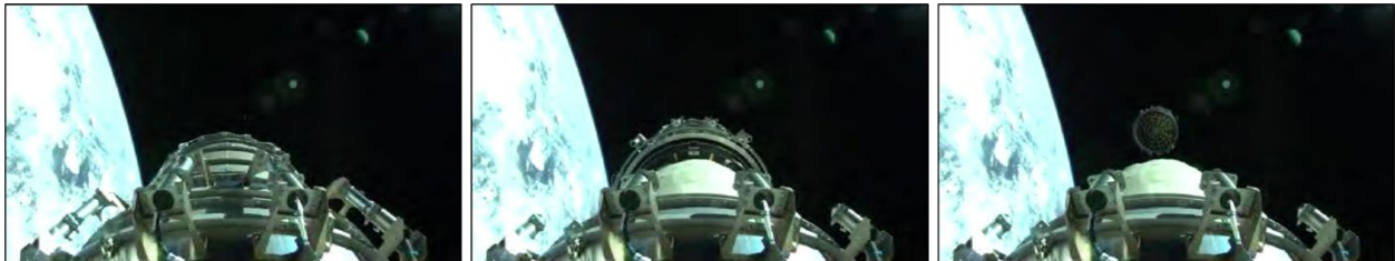
Figure 7: Payload Adapter Canister Jettison
