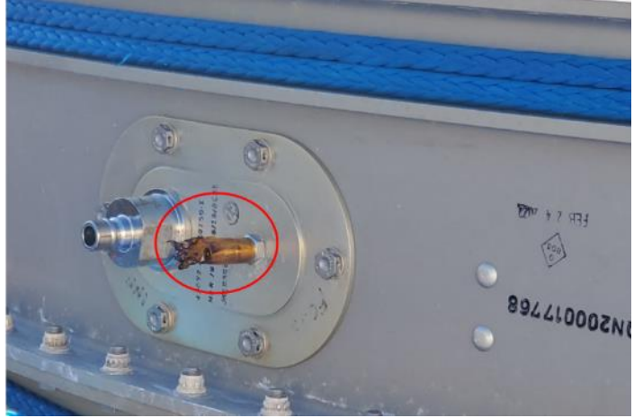
Figure 26 – Left is Blistered Tygon Tubing and Scorched Kapton Tape on RV Pair
