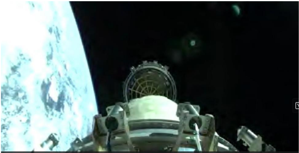
Figure 3 – A view of the PASS as the Payload Adapter moves away from LOFTID
