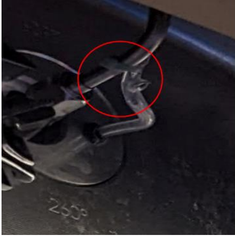
Figure 26 – Left is Blistered Tygon Tubing and Scorched Kapton Tape on RV Pair
