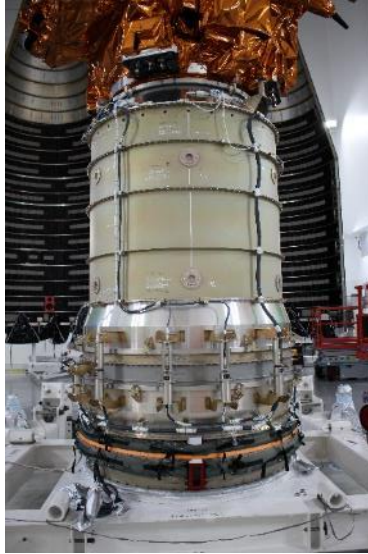
Figure 2 – Payload Adapter with JPSS-2 attached and LOFTID enclosed
