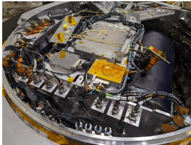
Figure 14 – Inflation System Installed in the Forward Segment
