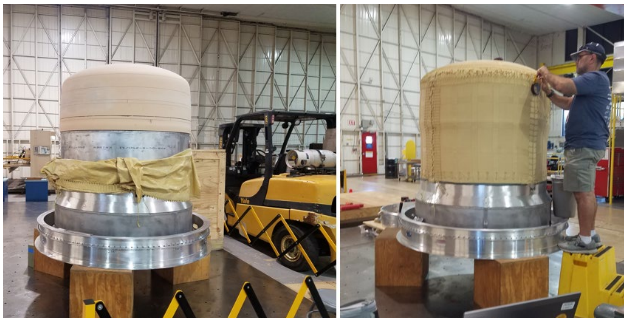
Fig. 15 RV Stand-In stowed aeroshell surrogate (left) with packing restraint EDU being installed (right).
