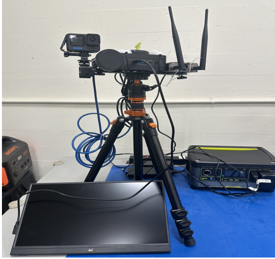
Fig. 4 Bench Setup of Camera Ground Node
