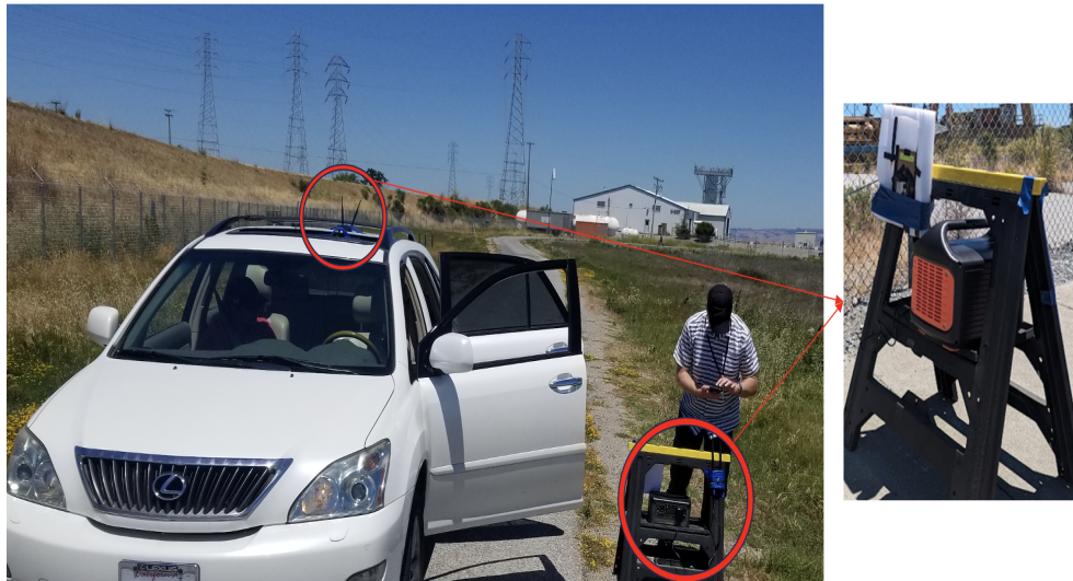
Fig. 31 Drive-Around Setup for the RF Mesh Modems
