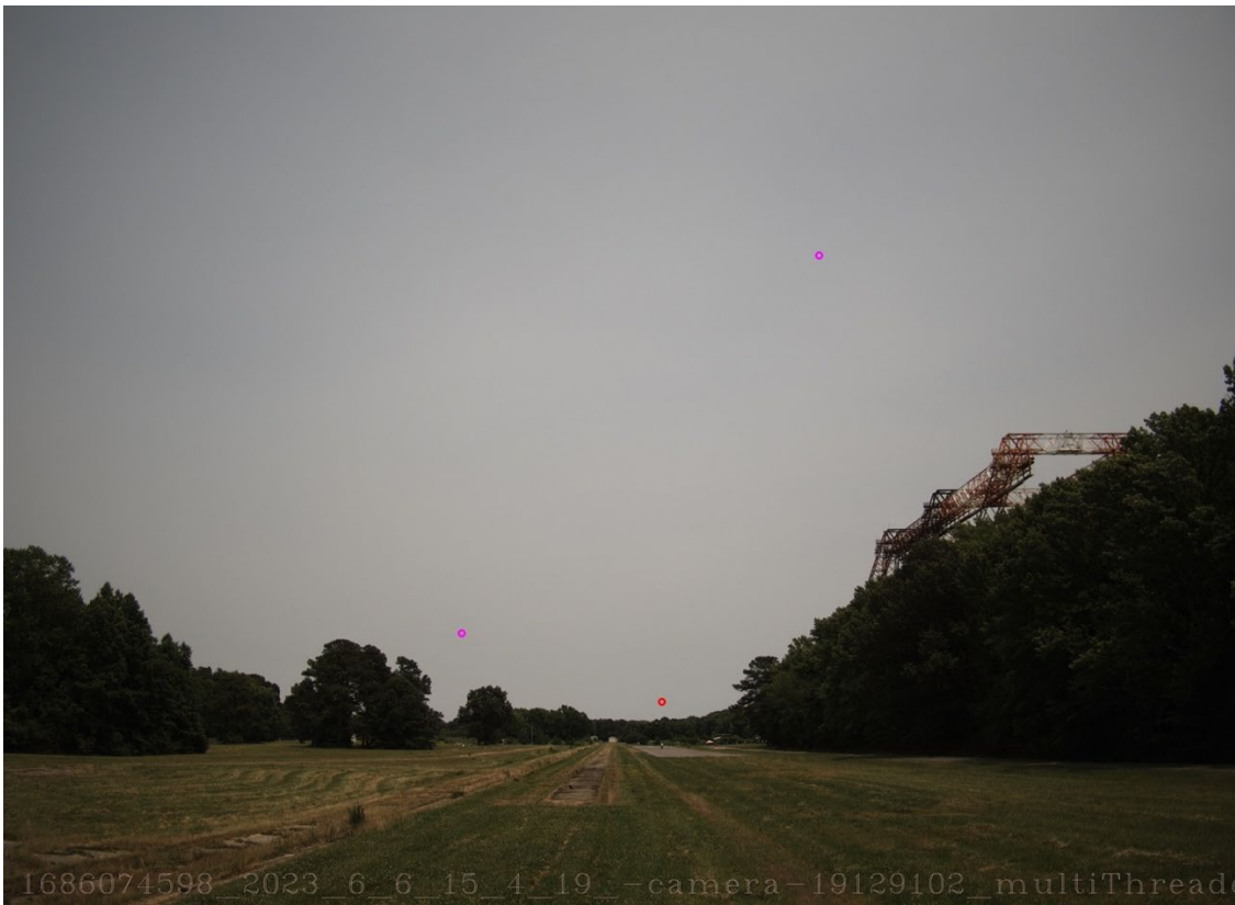
Fig. 11: Output of detection algorithm from [24] where red are morphological detections and magenta are image differencing detections. The bottom two detections are the HDV SUAS while the upper magenta detection is of an aircraft entering the flight area.
