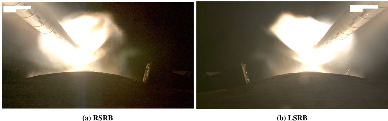
Fig. 4 Images captured by core stage cameras of the Artemis I booster separation event. Light from the engines illuminates a small number of photogrammetry points (e.g., black strips) on both boosters [photo: NASA].
