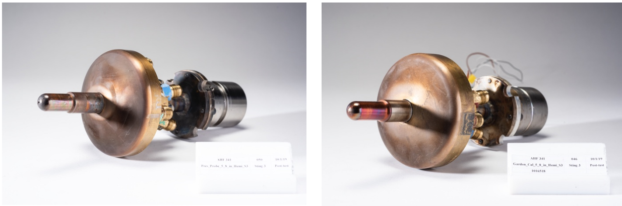
Figure 2. Photographs of the 1.59-cm hemisphere pitot probe and Gardon gage calorimeter used for the flow surveys in the TP3 15-inch and AHF 12-inch nozzles.
