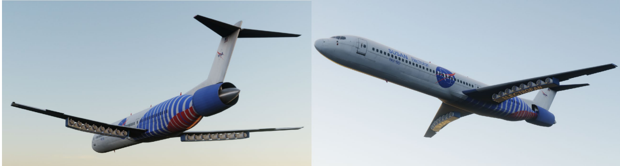
Figure 1.—NASA concept renderings of SUSAN Electrofan aircraft.
