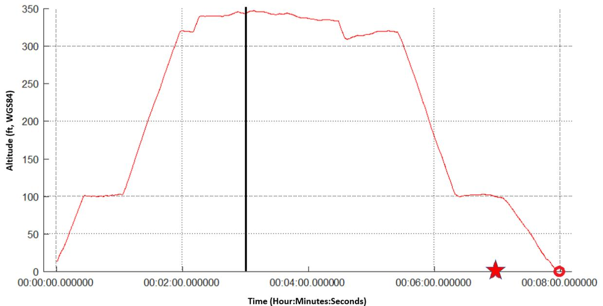
**Fig. 15 Altitude during speed change scenario.**
