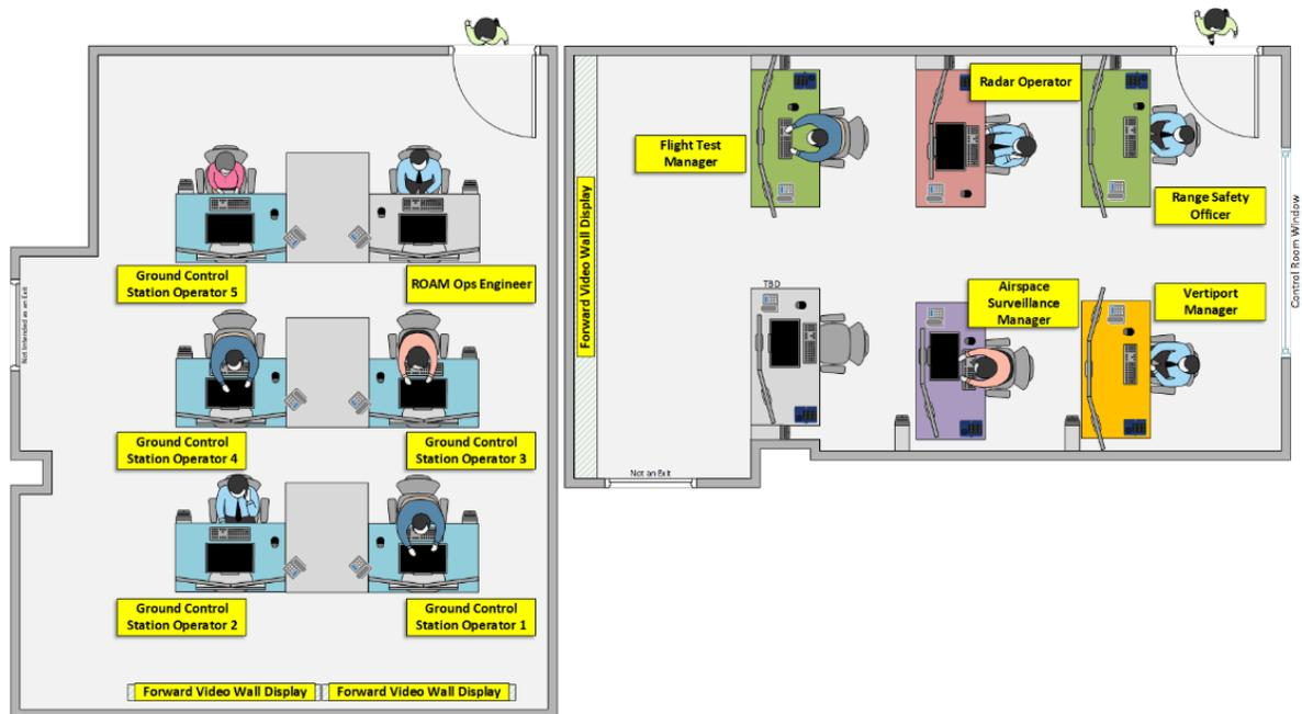
Fig. 1 Plan view diagram of ROAM Facility.
