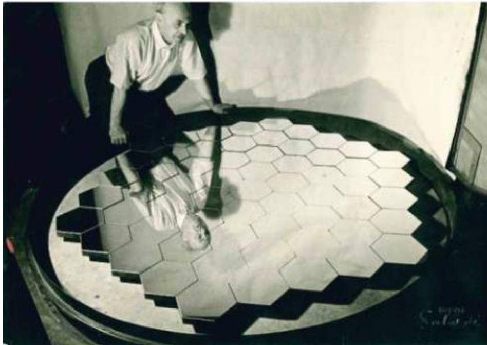
Guido with the completed 1.8-m segmented telescope with 61 segments in 1952 (credit: [13])
