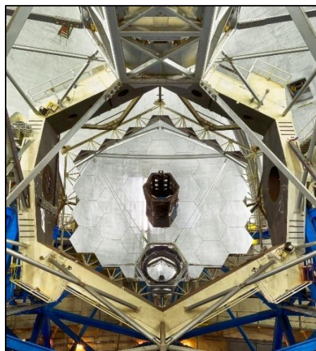
Left: Design of 10-m primary mirror with 36 segments. (credit: [15]) Middle: Keck mirror assembled. Right: Jerry Nelson “Father of the Keck telescope segmented-mirror design”. (credit: Keck Observatory Archives)
