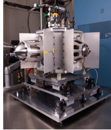
Fig. 12. Final Testbed assembly integrated on test stand
