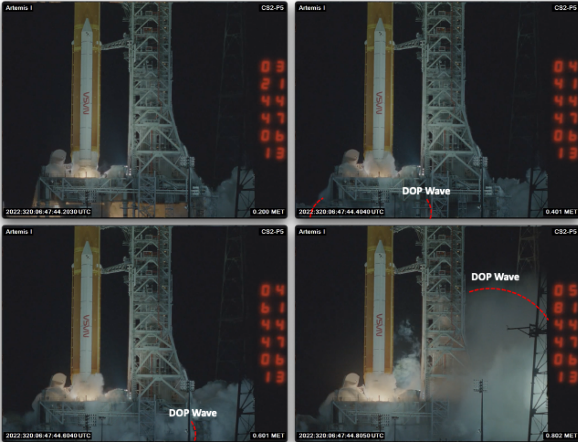
Fig. 4 Artemis I high speed video (images.nasa.gov) showing the DOP wave traverse and exit the flame trench.
