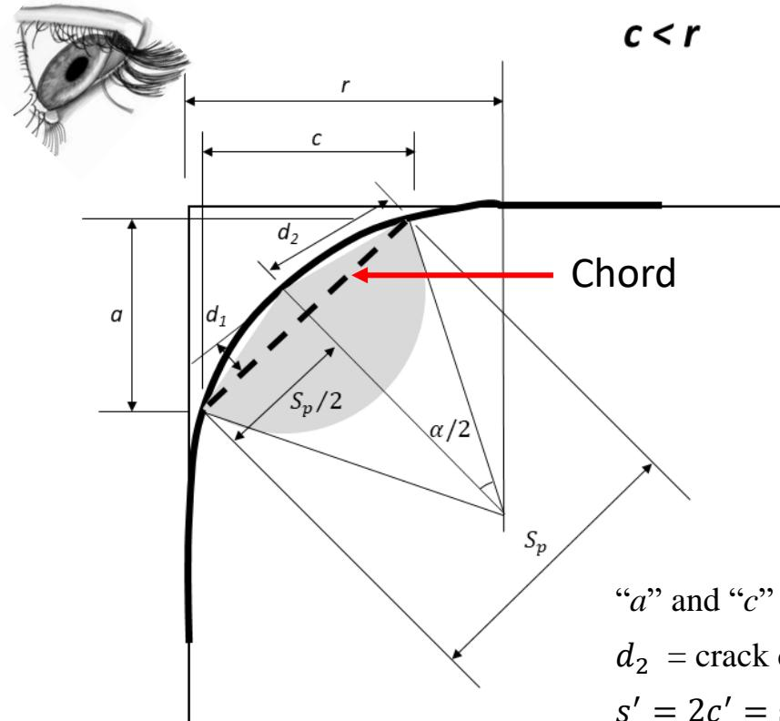
Chord length is perceived as dye penetrant indication length by the eye looking at the corner
