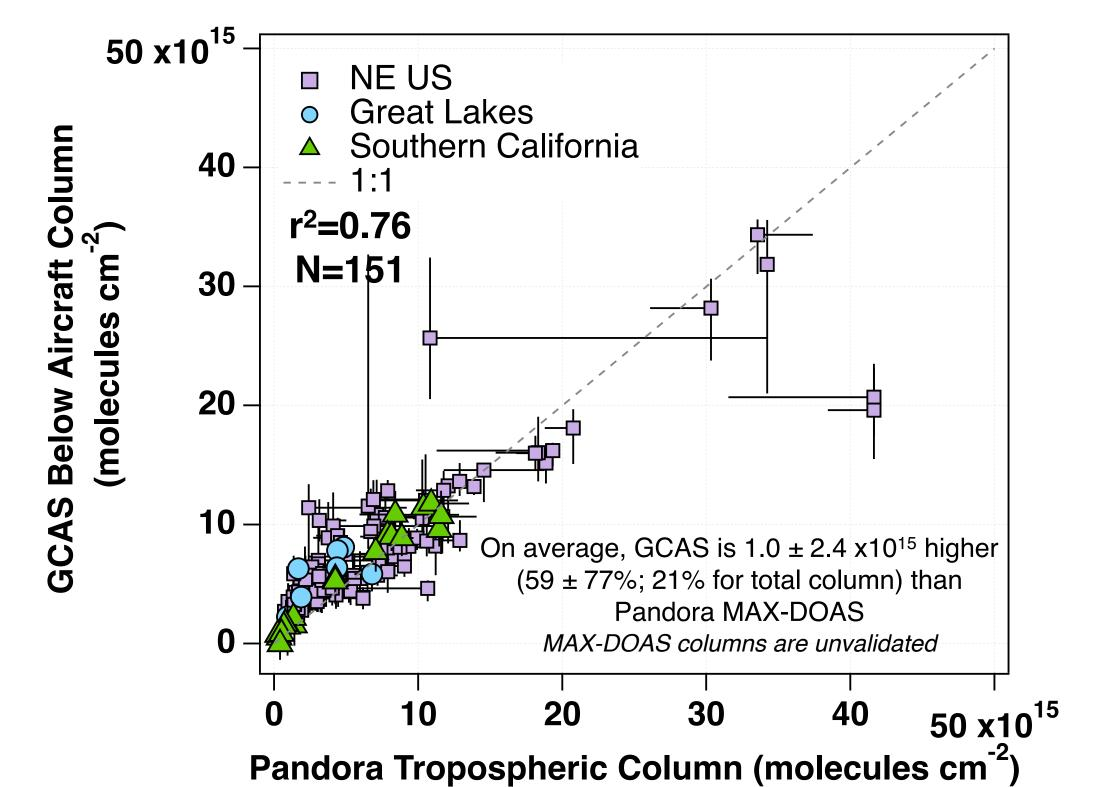
Plots show the median GCAS value within 750m of the Pandora site during the overpass. Vertical bars are the 25th-75th percentile within that 750m radius. The Pandora value is the nearest in time where the horizontal bars represent the max/min within 15 minutes of the GCAS overpass.
